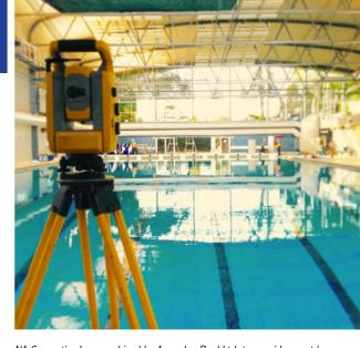
NA Geomatics Inc. was hired by Acapulco Pool Ltd. to provide exact lane dimensions and 'parking' positions for new bulk-heads in the Canada Games Aquatic Centre. NA Geomatics Inc. used a S3 robotic total station to undertake the necessary tasks.
